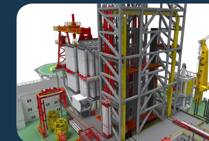
Drilling in Ram Rig-port & running casing in Ram Rig-Starboard
