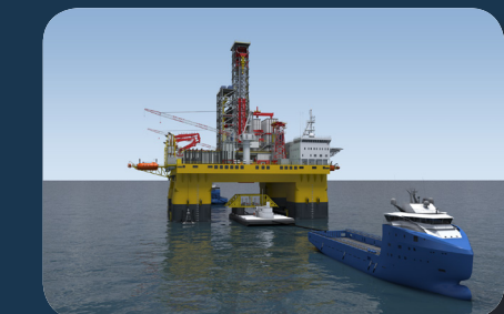
Barge with template positioned under rig with AHV's
