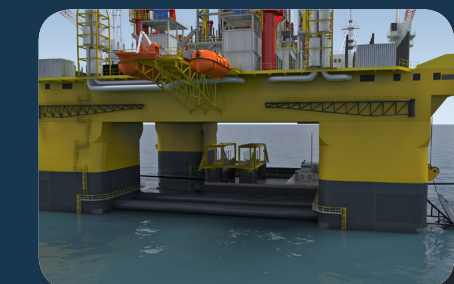
Heavy loads lifted off barge and lowered into water
