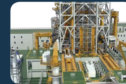
Drilling in Port-Rig & running casing in Starboard-Rig
