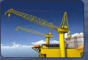
SUPERB LOGISTICS Two (2) 50 MT Deck Cranes with 45.8m boom covering most of the deck space and good coverage on the wellheads/jackets.
